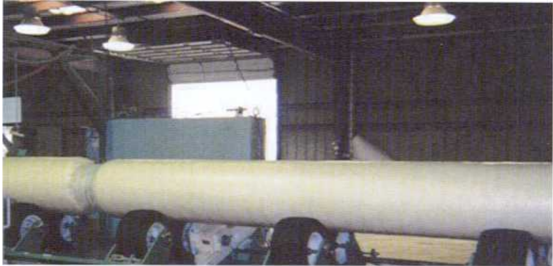
XTRU-THERM insulation prior to the application of the seamless HDPE jacket
